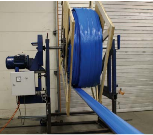
winding of a long length on a wooden reel
