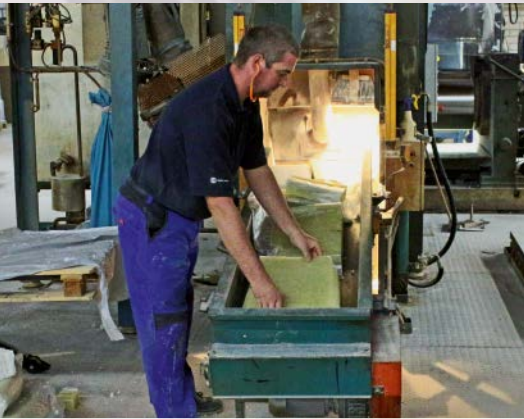
an employee places the pre-weighed mixture components to the conveyor belt, which transports the components in the internal mixer
